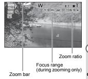
Once the button is released and pressed again, the camera switches to digital zoom.
